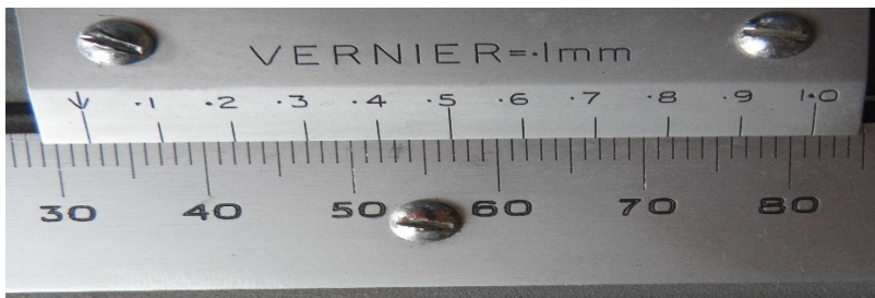
Figure 2 - Vernier scale reading 32.4 mm
